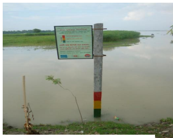
Flood Level Scale. By seeing water level, people can measure danger of flood. ©RDRS Bangladesh
